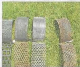
Different blades are used to vary the consistency of corn into corn meal.
